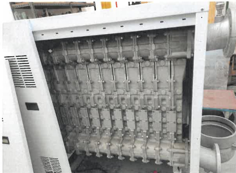
Photo of heat exchanger
